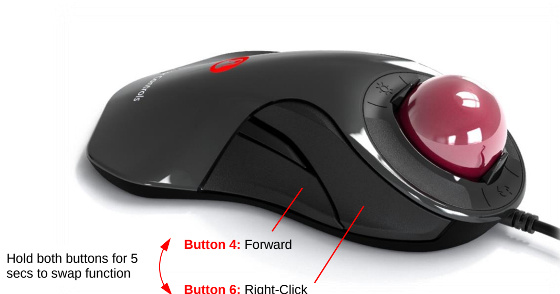
Figure 7: Right/Forward Button Configuration***
